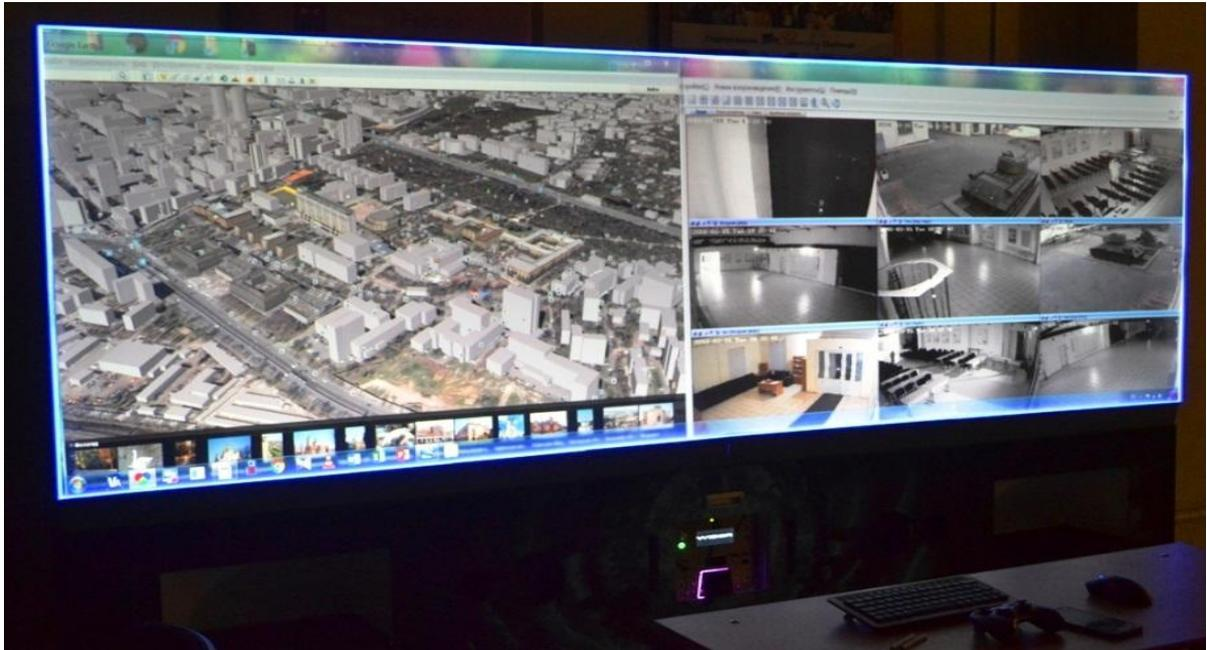
The device is a projection monoblock with onboard media server, sound system, uninterruptible power supply and provides the ability to connect both external and local equipment, as well as storage devices and workstations.
